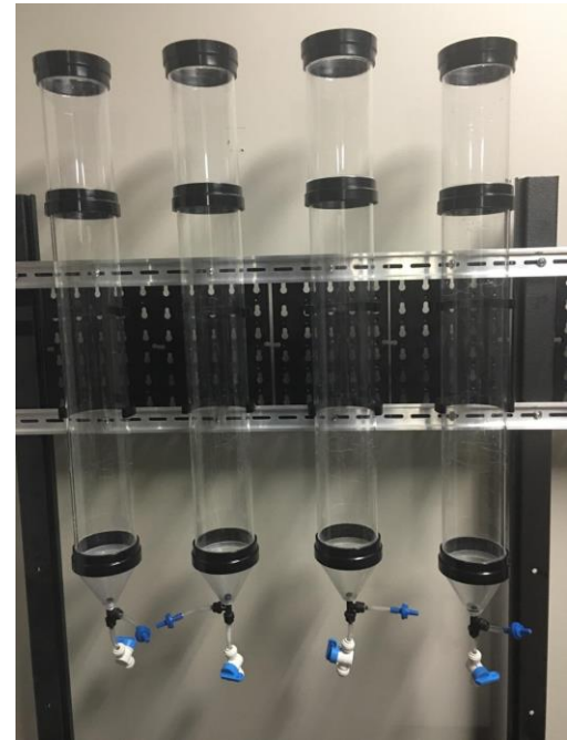
Fig 4. Lab scale airlift being developed at FSU
